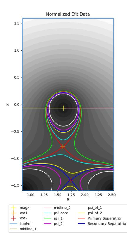
**Warning:** When setting use\_efit\_bounds to True, the user must provide a non-zero value for values efit\_buffer\_r and efit\_buffer\_z.
