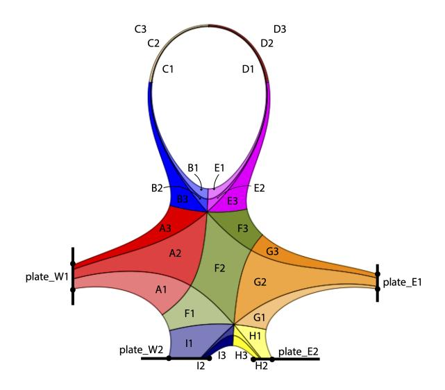
The user should reference the above figure when prepping the parameter file for generating a Patch map by verifying target plates are in valid locations relative to x-points and psi-boundaries.
