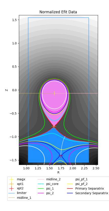
To emphasize the dependence on the limiter for decomposition, we also illustrate with setting both  $efit_buffer_r$  and  $efit_buffer_z$  back to their **default** values of 1.0e-2.
