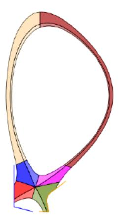
**Tip:** Applying these Patch modifications appropriately can allow one to increase cell density near primary x-point without modifying np/nr values
