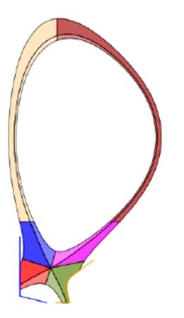
In a similar manner to adjusting the angle of line tracing in the E and W directions from the primary x-point, we can adjust the line segments extending from the magnetic-axis. These line segments define the east faces of patches B1 and B2, as well as the west faces of patches E1 and E2.
