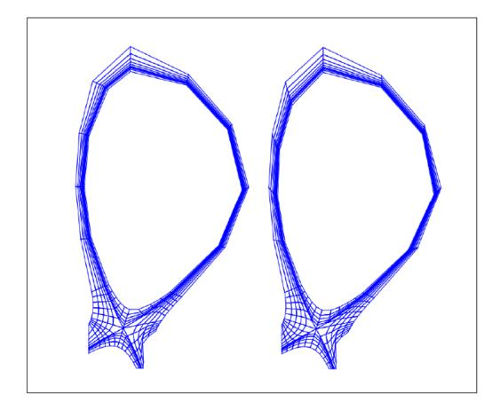
We can see that the radial lines are indeed more orthogonal to the poloidal contours. Although only a mild effect in this case, we have seen that distortion\_correction can significantly reduce shearing and generate tidier grids in others (example SF cases seen below).
