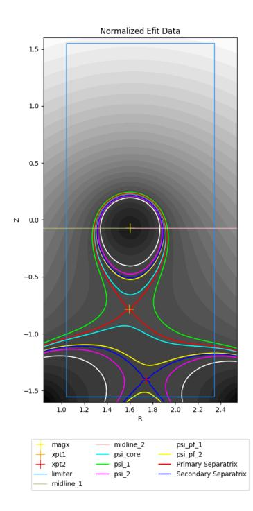
We can immediately see the presence of a secondary x-point, it's corresponding separatrix, a rectangular (psuedo) limiter and additionaly psi lines that we will use to generate a Patch map.
