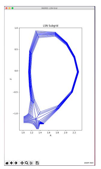
We can continue to modify the grid in order to allocate more cells near the x-point. A natural choice would be to target  $np_B$  and  $np_E$ . Doing so with the values  $np_B = 18$  and  $np_E = 18$  (double resolution for the larger patches), we see our parameter file consists of:
