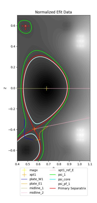
Immediately we see that there is a line segment originating from the primary x-point and extending to the EFIT domain boundary.
