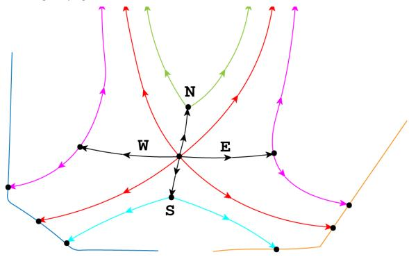
Tracing in direction N, S, E, W are orthogonal to flux surfaces.
