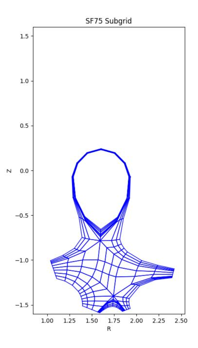
Using np\_default and nr\_default with values of 3 produces the following grid when using the limiter.
