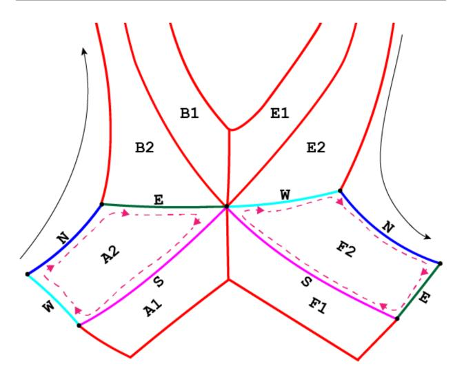
The **N** boundary (seen in dark blue) for Patch A2 begins at the max-psi strike-point on the target plate west of the primary x-point (inner target plate for SNL case), and terminates at the B2 interface. The **S** boundary (seen in magenta) for Patch A2 is oriented in the opposite direction and terminates upon intersection with the target plate.
