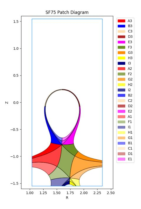
All grid generating instructions detailed in the SNL case also apply to the SF cases. The only difference is the addition of an additional control  $nr_3$  that controls the Patch objects with name ending with 3.
